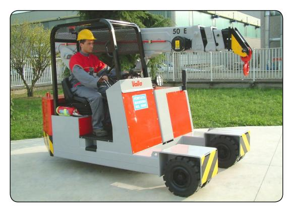
**DRIVE:** by DC 7 kW - 48 V fanned reversible electric motor with MOSFET electronic control HF and energy saving, self diagnostic, speed and temperature checks (no. 2 thermostasts), brush wear warning. Foot hydraulically operated brake to drive wheel. Hand brake mechanically operated. Gear box between motor and drive wheel in oil bath. Speed up to 8 km/h.
